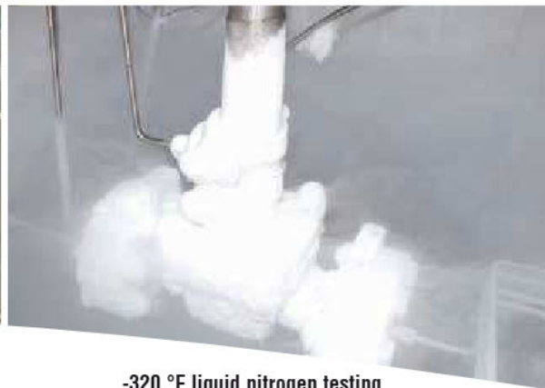
-320 °F liquid nitrogen testing
